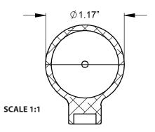
Commercial receiver extensions have a slightly larger diameter of 1.170", and sometimes have slanted backs. Only the Commercial CTR will slide easily over this tube. **Do NOT force a Mil-Spec CTR over a commercial tube!**
