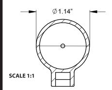
Mil-spec receiver extensions have a slightly smaller diameter of 1.146," and have a flat back. Both the correct Mil-Spec CTR and the Commercial CTR will fit over this tube, but the Commercial CTR will be loose.
