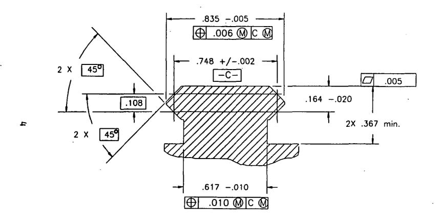
FIGURE 1. Accessory mounting rail profile
