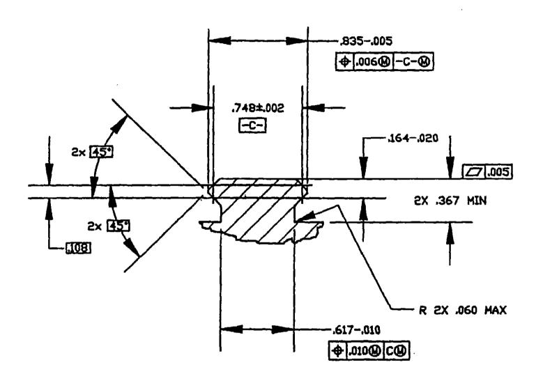
FIGURE 1. ACCESSORY MOUNTING RAIL PROFILE
